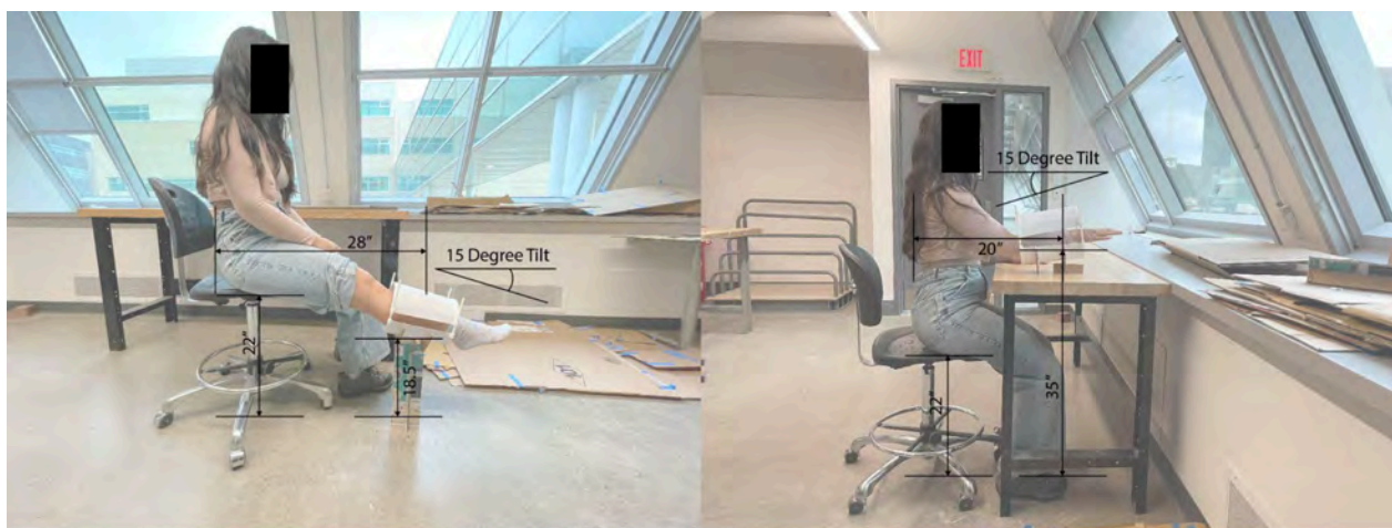
PORTABLE CASTING MACHINE 1:1 SCALE MODEL ERGONOMIC STUDY 50% FEMALE 95% MALE
