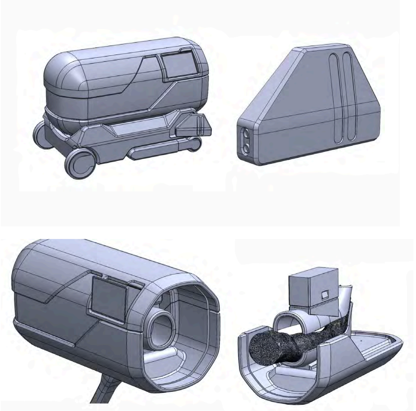
Figure 62: CAD Development: Material Canister, Display Release, Auto Casting
