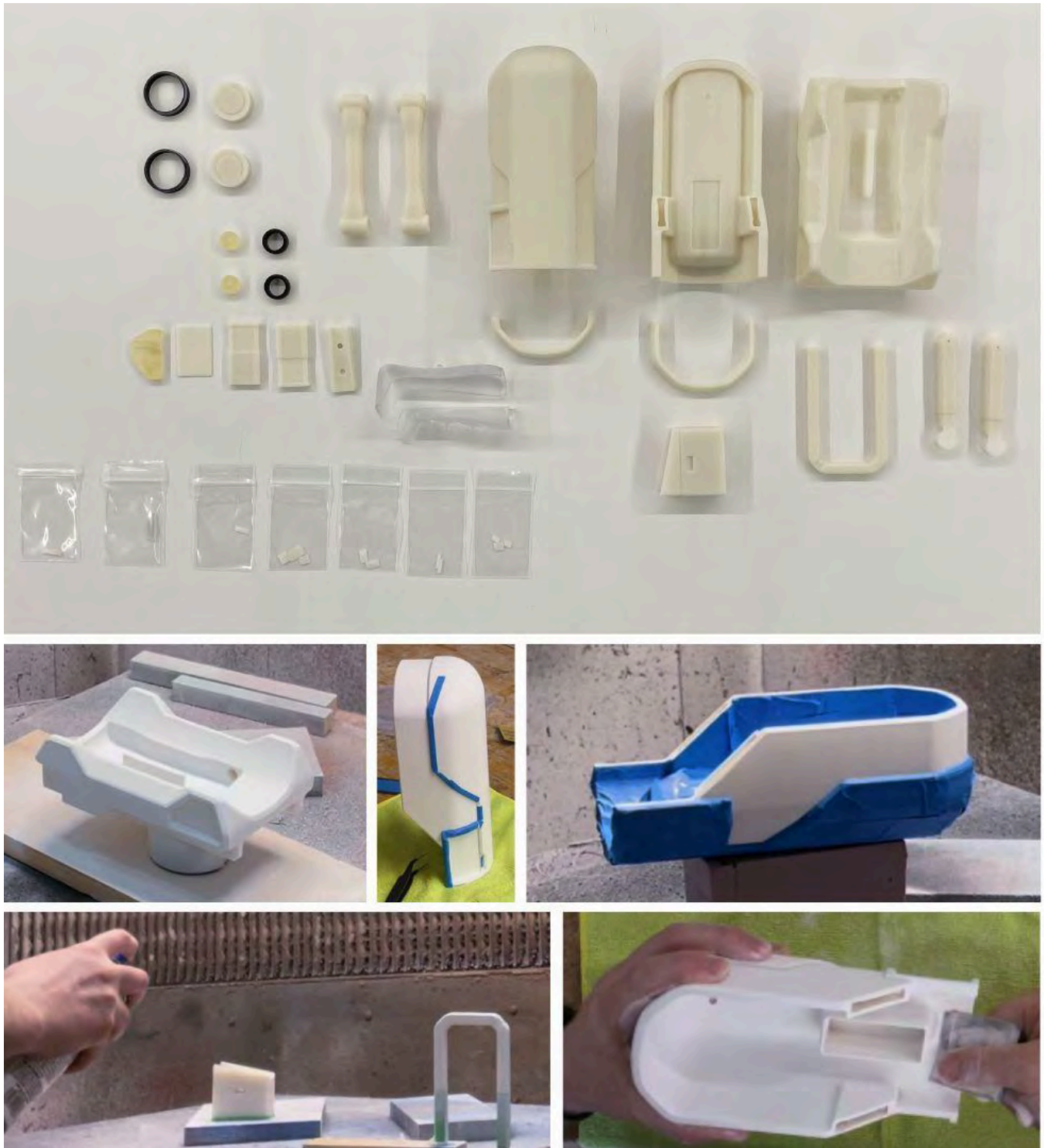
Figure 64: Physical Model Fabrication: Printed Parts, Sanding, Painting, Masking
