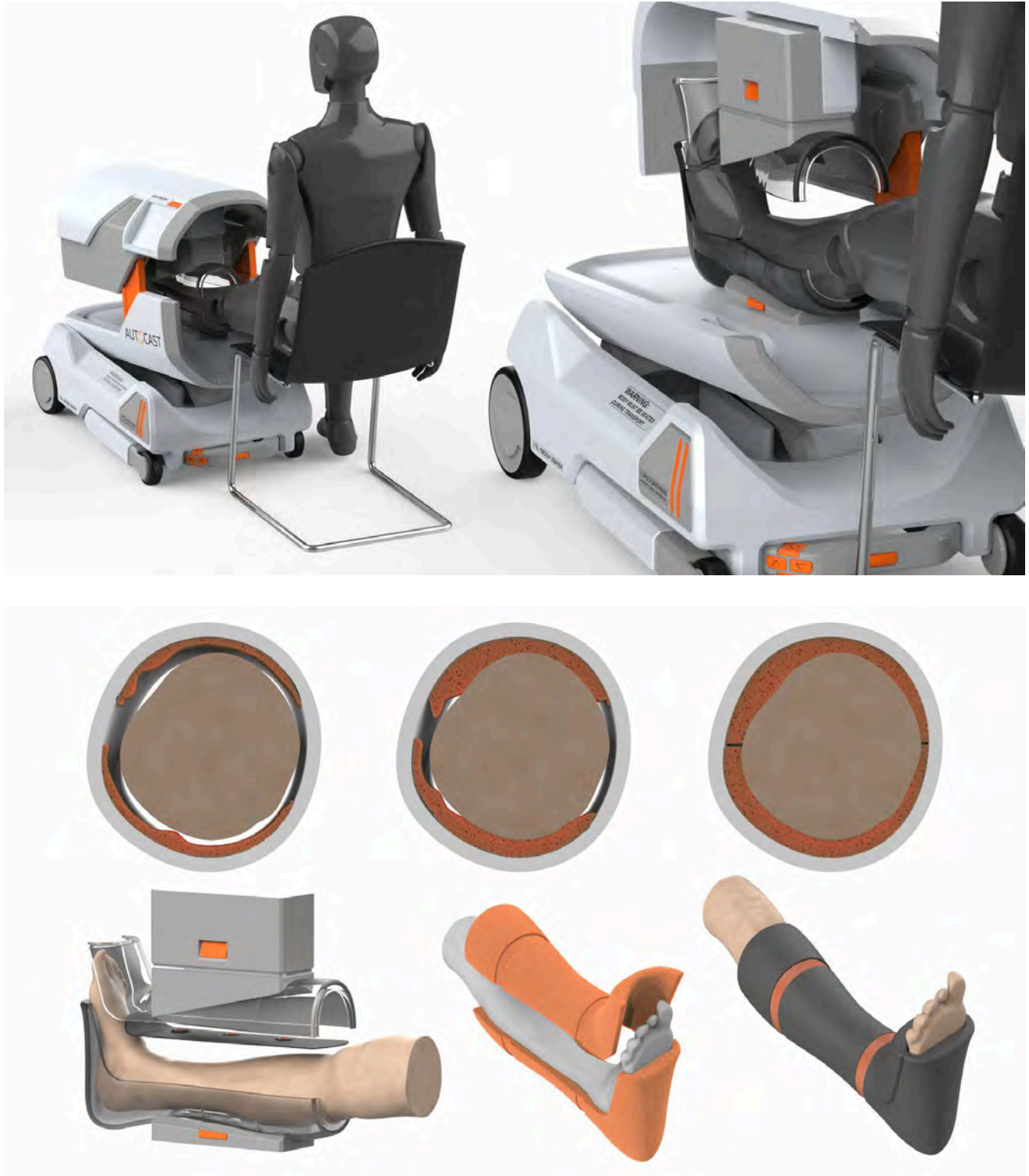
Figure 72: Final CAD Rendering:Automatic Cast Applicaiton, Material Expanding around patients limb.
