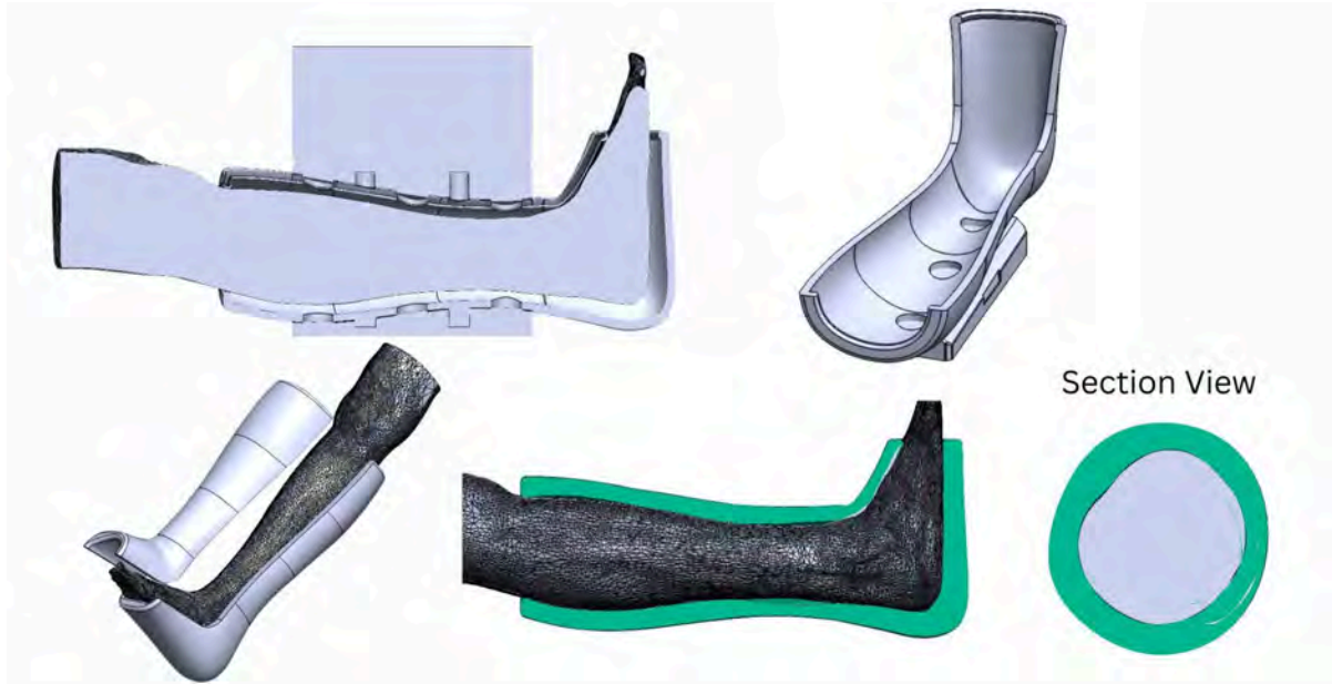
Figure 63: CAD Development: Cast Mold, Cast Procedure, Bi-Valve Cast
