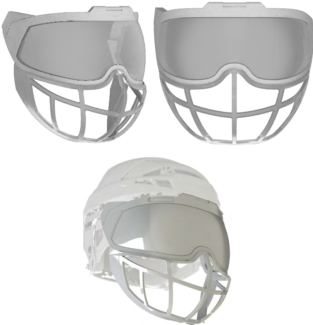
Figure 22 – CAD Development for face shield including helmet 3D scan
