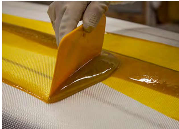
Figure 4: A worker spreads resin onto layers of fibreglass underneath. Image source: Fibre Glast Developments Corp.
