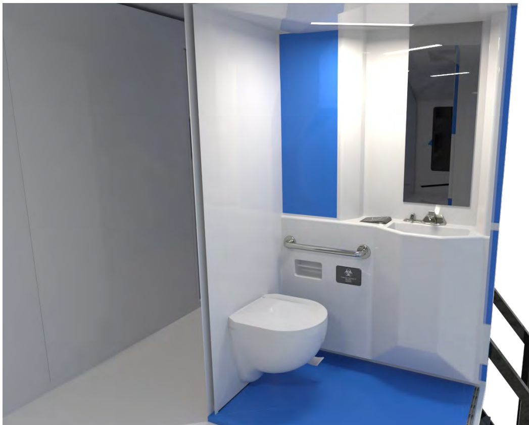
Figure 67: Final render of toilet stall. Walls have been cut to better view inside.
