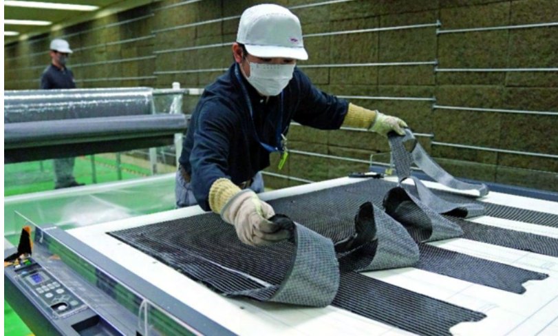
Figure 3: A worker lays sheets of carbon fibre onto a surface, in a process similar to that of fibreglass.
